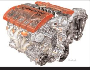
DOWNLOAD | X06PT\_AR003 The production 7-liter LS7 engine that powers the 2006 Z06 Corvette produces 505 horsepower, the highest output of any GM small-block V-8.
